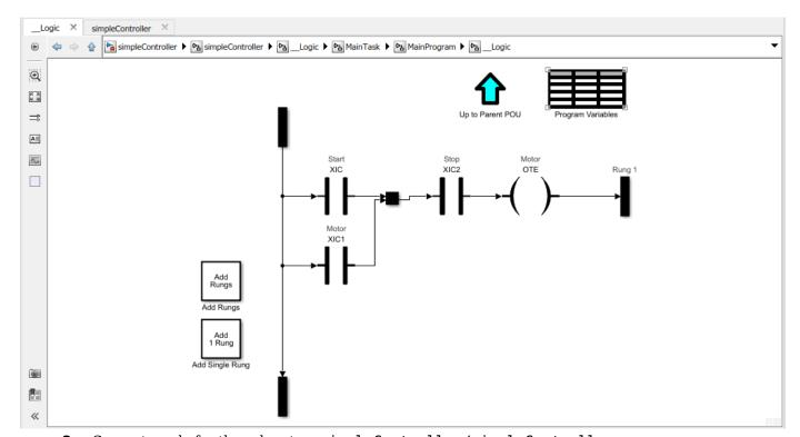
**3** Generate code for the subsystem simpleController/simpleController.
