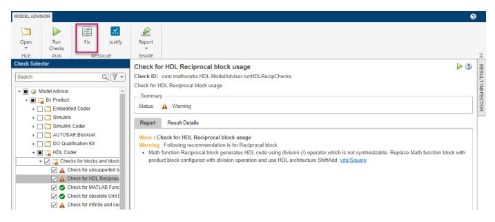
When you select **Fix**, the **Action Report** window shows the changes that were applied. To verify that the check passes, rerun the check.
