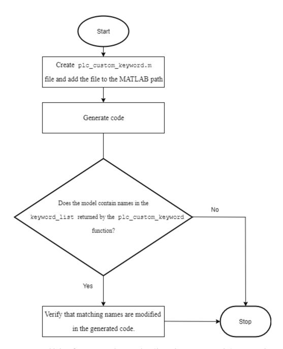
You must add the plc custom keyword.m file to the MATLAB path for custom keyword checks to work.
