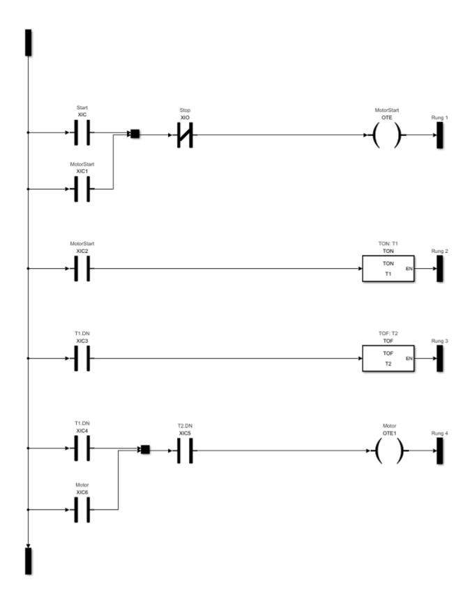
This ladder logic has a TON timer named T1 that is responsible for the delay when starting the motor. The ladder logic has a TOF timer named T2 that is responsible for the delay when stopping the motor. T1 has a preset of 5 seconds and T2 has a preset of 10 seconds.
