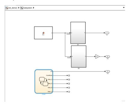
The S1 and S2 blocks are identical and contain a simple feedback loop. The Stateflow chart contains a simple state machine.
