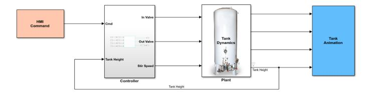
This model is the completed model for the ladder tank controller example. The controller is autogenerated from the ladder file TankControl.L5X by using the plcimportladder command.
