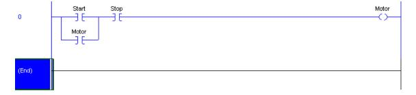
1 Use the plcladderimport function to import the ladder into Simulink.
