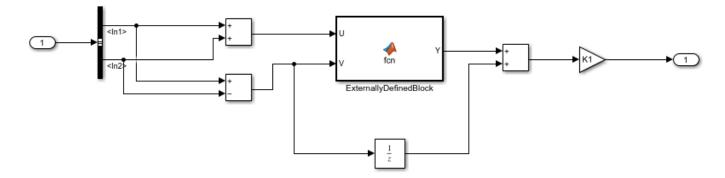
To do this, right click on the top level subsystem 'Subsystem' and select 'PLC Code -> Options ...' to bring up the 'Configuration Parameters' dialog box. In the dialog box, select 'Symbols' pane under 'PLC Code Generation'. You will see the following symbols in the 'Externally Defined Symbols' field:
