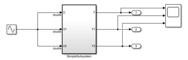
This model shows the usage of tunable parameters by specifying them as Simulink.Parameter objects in MATLAB base workspace. This model makes use of three parameters K1, K2 and K3 defined in the MATLAB base workspace as Simulink.Parameter objects (please see 'setup\_tunable\_params.m' in the same directory as this model).
