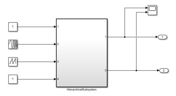
This introductory model shows the code generated for a hierarchical subsystem consisting of two other subsystems named "S1" and "S2". These subsystems are not marked atomic and hence they do not generate separate Function Blocks. The code for these subsystems gets inlined into the Function Block for the parent subsystem "HierarchicalSubsystem".
