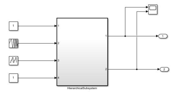
This introductory model shows the code generated for a hierarchical subsystem consisting of two other subsystems named "S1" and "S2". Each of these subsystems generate a separate Function Block. To build the subsystem, right-click on the subsystem block and select PLC Code > Generate Code for Subsystem.
