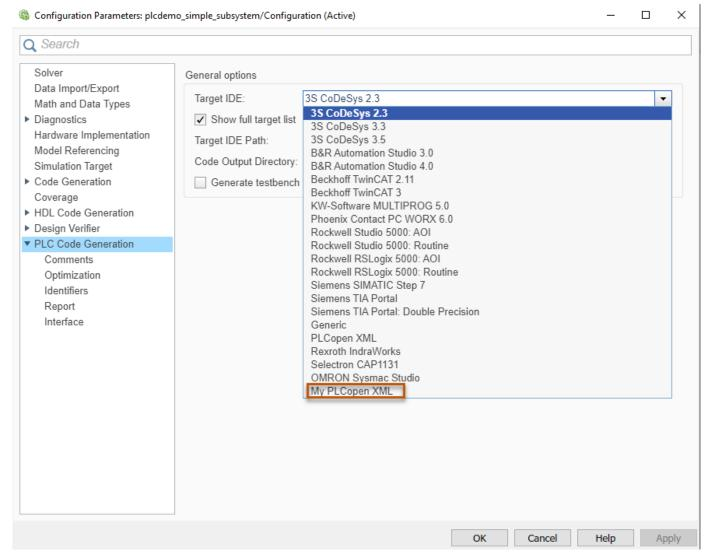
7 In the PLC Code app, PLC Code tab, click Generate PLC Code to generate code for your custom target IDE. The generated code files are placed in the path specified in ide\_info.path = ''; % IDE path.
