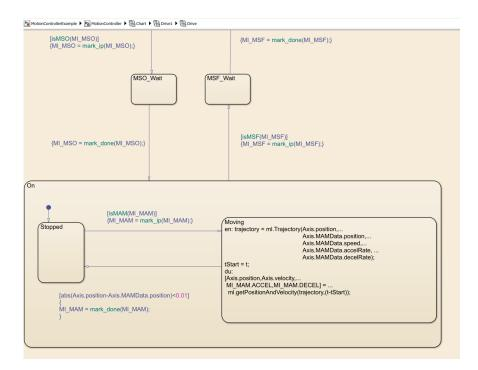
The drive logic Stateflow chart models a real world drive with parameters such as trajectory and delay. Any drive subchart has this data:
