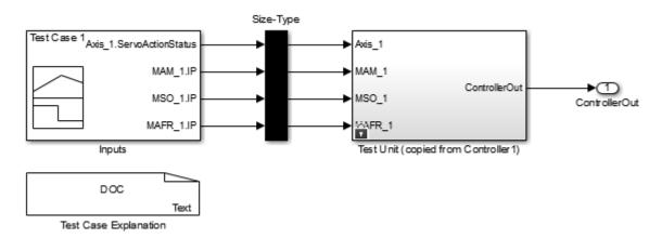
• Open the Inputs block in the test harness model. The Inputs block is a Signal Builder block that can have one or more signal groups.
