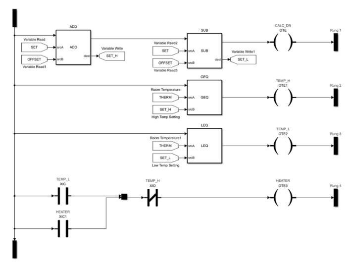
The first rung calculates SET\_H and SET\_L. On the second rung, when the room temperature is greater than or equal to SET\_H, OTE1 is on. On the third rung when the room temperature is lesser than or equal to SET\_L, OTE2 is on. When OTE2 is on and OTE1 is off, the heater is on.
