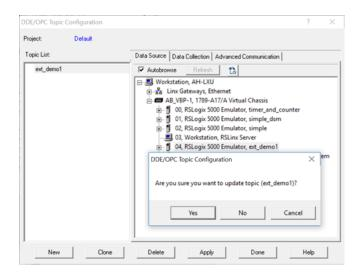
To verify the OPC server setup, in RSLinx® select **Edit > Copy DDE/OPC Link**. If iO\_Subsystem\_val is present, the server configuration is complete.
